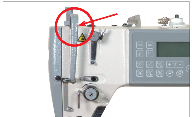
挑線杆在高點 Retainer at the highest point
